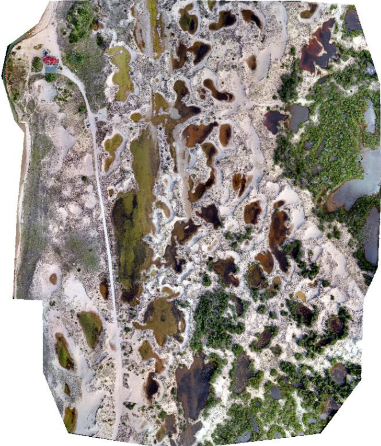
Figure 9. Orthomosaic of study area created from UAS imagery, 2019a (3 cm spatial resolution).
